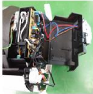
Disconnect PCB connector before completely removing Discharge assembly.
