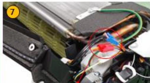
Disconnect PCB connector before completely removing Discharge assembly.
