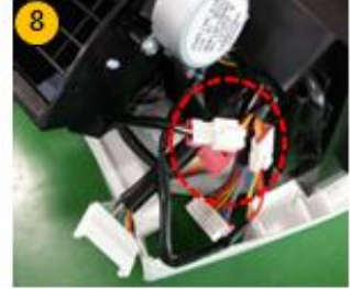
Disconnect PCB connector before completely removing Discharge assembly.
