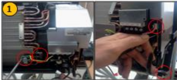
❖ Make sure to disconnect all the wire connections, sensors etc. from Control Box
