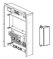
Step 2. Assemble the cover of independent power module, fix it tightly with bolts and connect wires.
