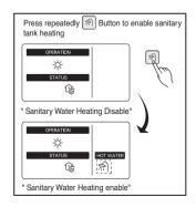
• Function Code 28 and 29 : Setting control parameter for Sanity water heating operation
