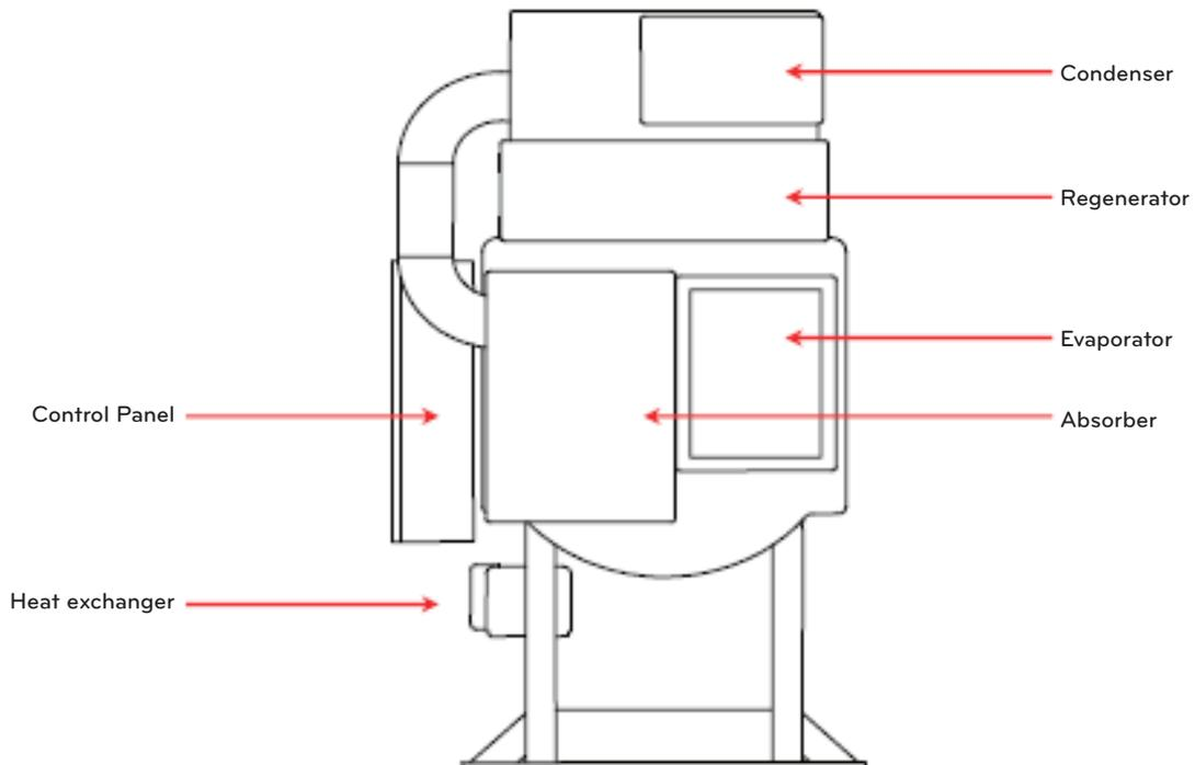
Figure 1-9 Rear view of main body
