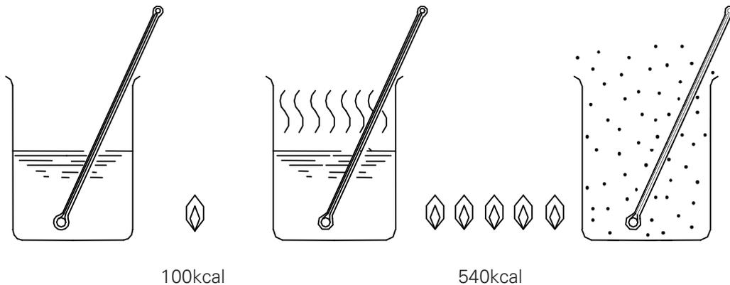
As shown above, using heat of vaporization rather than sensible heat, generated from 1kg (1ℓ) water, can transfer much more heat capacity. And water is normally evaporated at 100°C. But it can be evaporated at a lower temperature when air pressure is lowered. It is the reason why rice is half-cooked on a high mountain.
