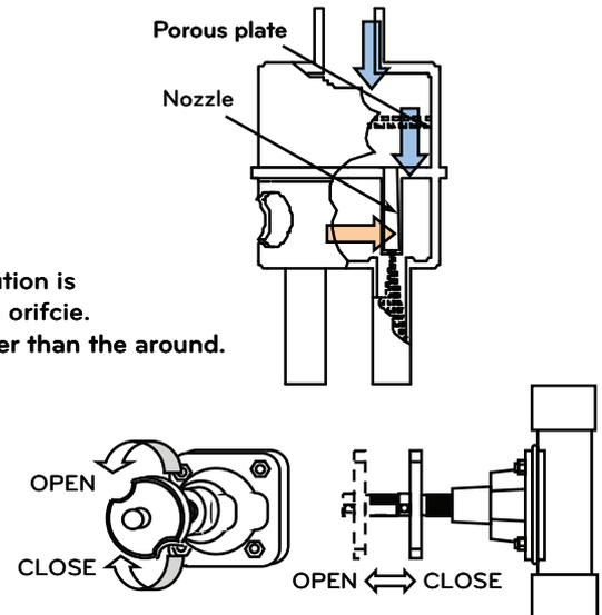
Figure 3-5 Purge valve (Diaphragm valve)
