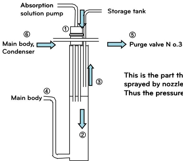
Figure 3-4 Storage tank and the principle of purging
