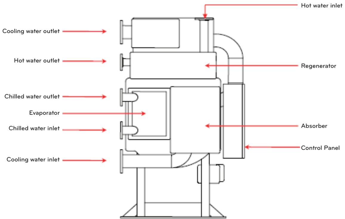
Figure 1-8 Front view of main body
