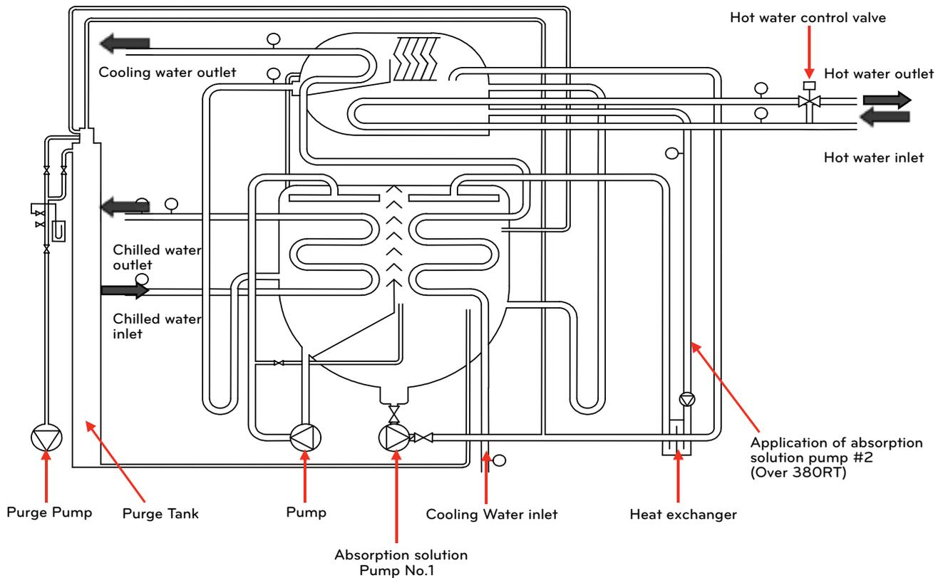
Figure 1-17. Layout of hot water type absorption chiller
