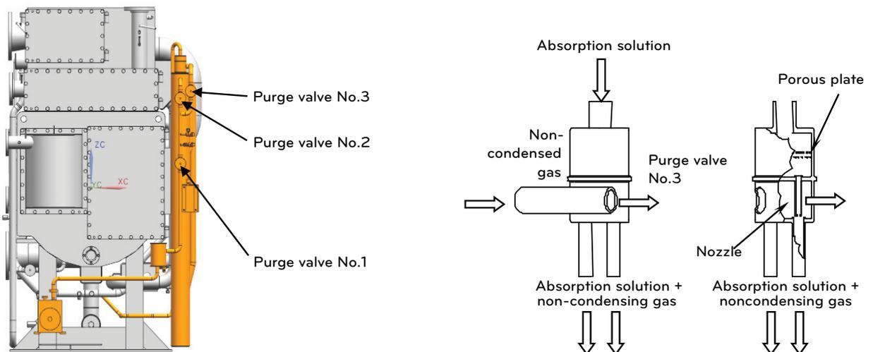
Figure 3-3 Structure of purge unit
