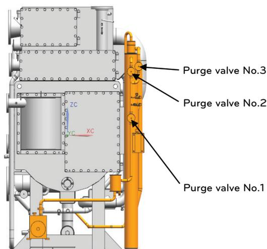
Figure 3-10 Structure of purge unit
