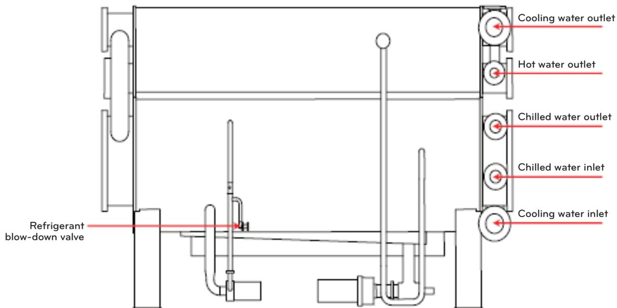
Figure 1-11 Side view of main body (Evaporator side)
