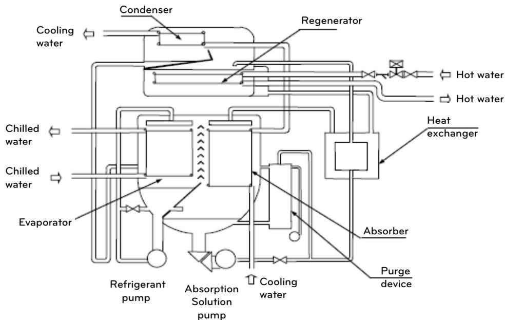
Figure 1-4. Basic cycle of absorption chiller
