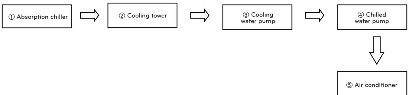
Figure 2-1. Startup and stop sequence of auxiliary equipment
