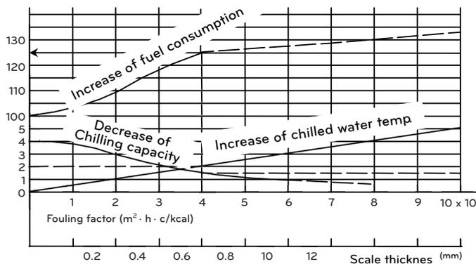
When scale is accumulated up to 0.6mm in the tube, cooling power goes down to 76% and the chilled water temperature rises up by about 2°C. And fuel consumption ratio increases by 25%.
