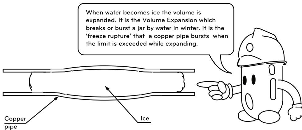
Figure 5-2 Freeze rupture
