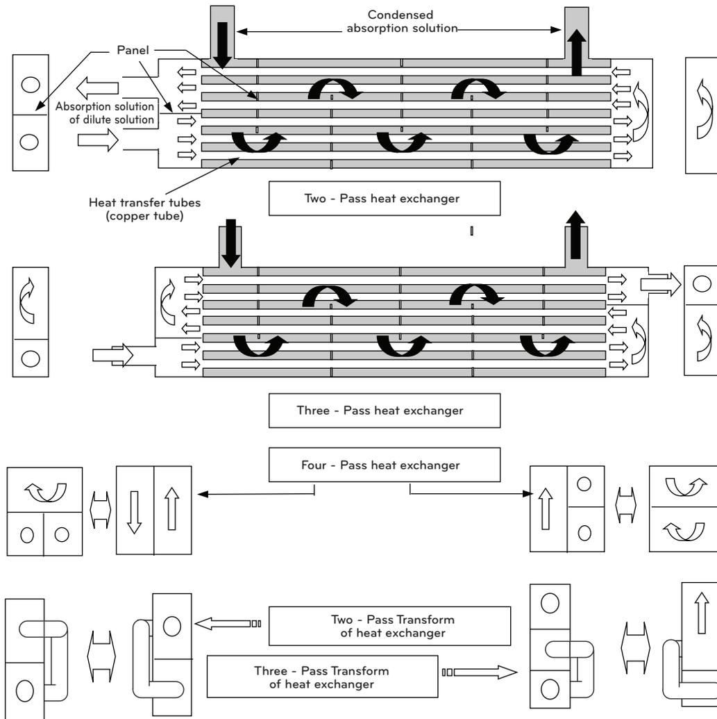
Figure1-16. Heat exchanger
