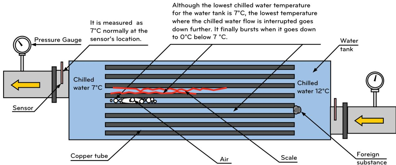
Figure 5-3. The cause of copper tube burst
