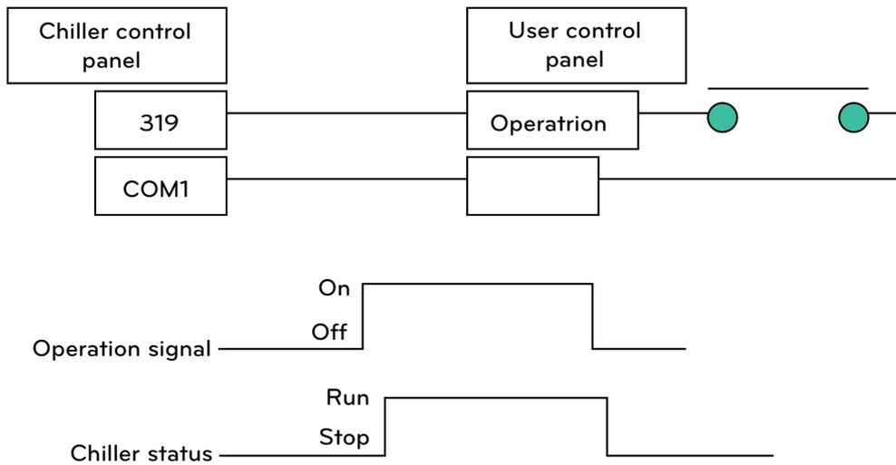
\* The minimum keeping time of run/stop pulse: Min. 2 seconds.
