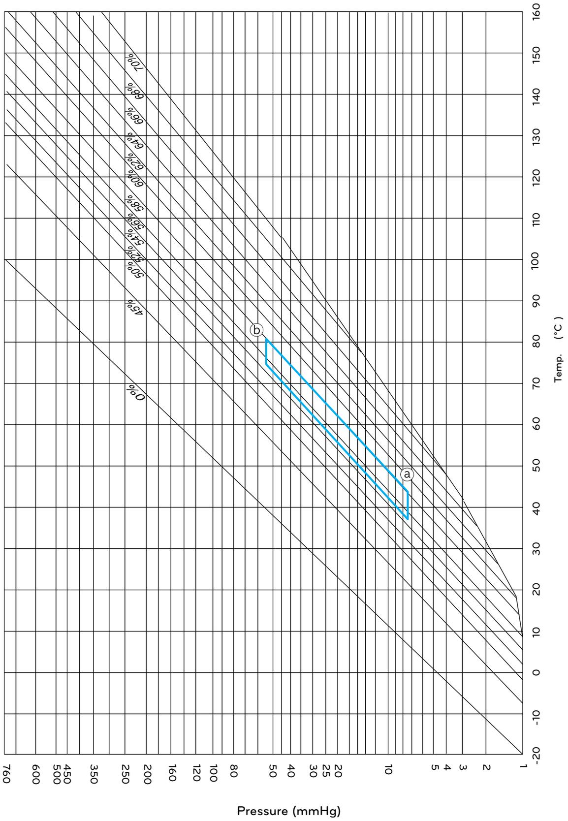
Figure 1-3. Duhring diagram
