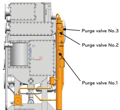
Figure 3-11. The structure of the purge unit
