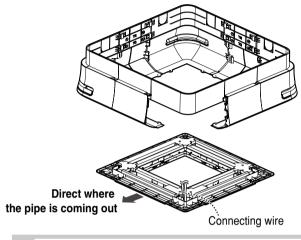
After selecting the direction you want, make holes for pipe and drain hose to fit the installation environment.
