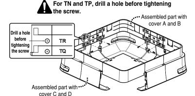
Check the direction of the front panel and set the cover on the panel. (The direction the connecting wire is coming out is the same as the location of the detachable cover.)
