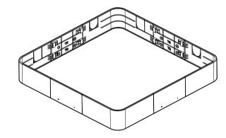
Assemble the remaining 3 covers C and 4 covers D so that they form a rectangular shape as shown in the picture.
