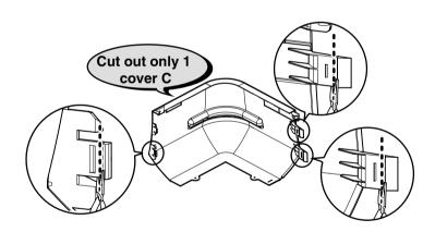
Assemble using cover C and D as shown in the picture and use the provided screws to tighten the covers. (6 locations)
