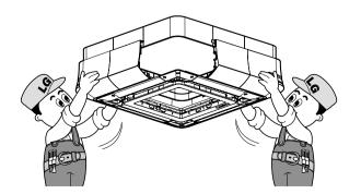
Use the provided screws to assemble the cover on the front panel. (14 locations)
