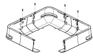
Complete the assembly until the rectangular shape is formed as shown in the picture.
