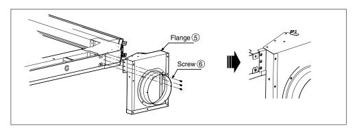
5-2. Use screws (6) to fix 4 points on the upper surface of the flange (5).
