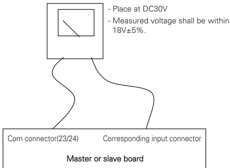
Figure 79. Master or Slave Board Current Measurement Circuit
