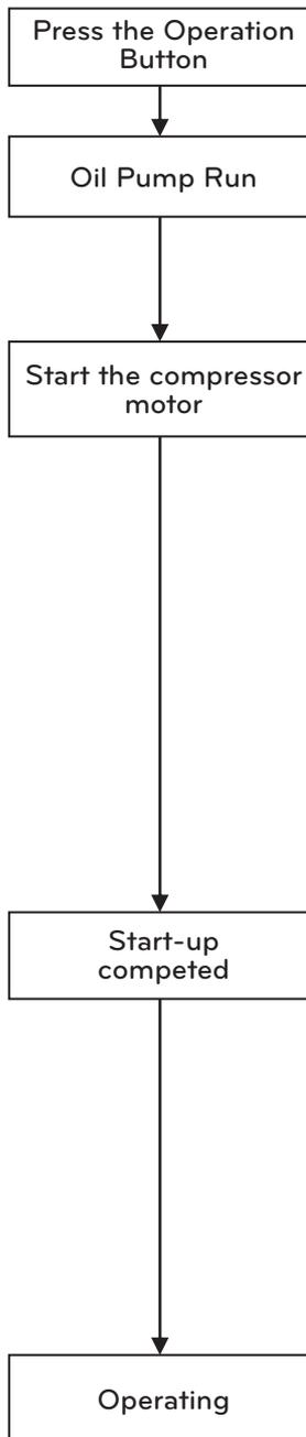
Figure 60. Test run procedure (2)
