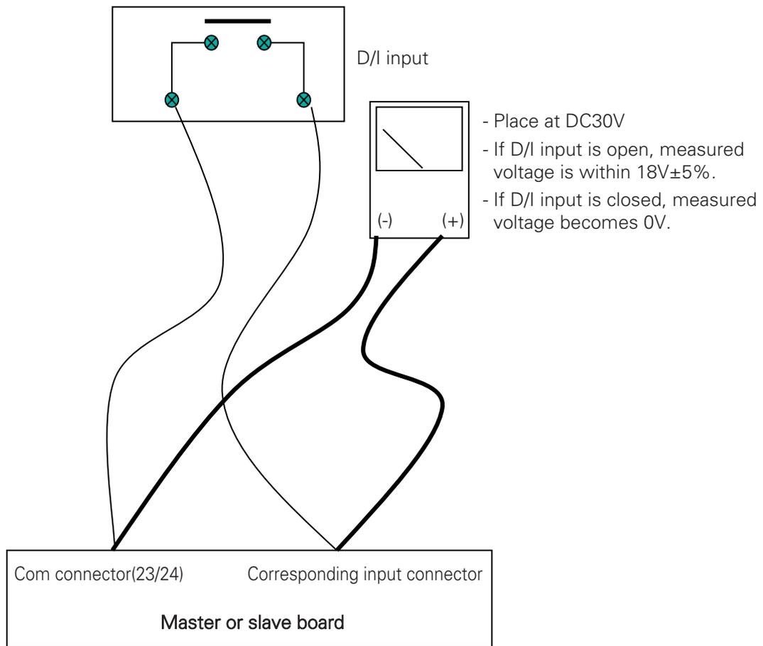
Figure 78. Master or Slave Board Current Measurement Circuit
