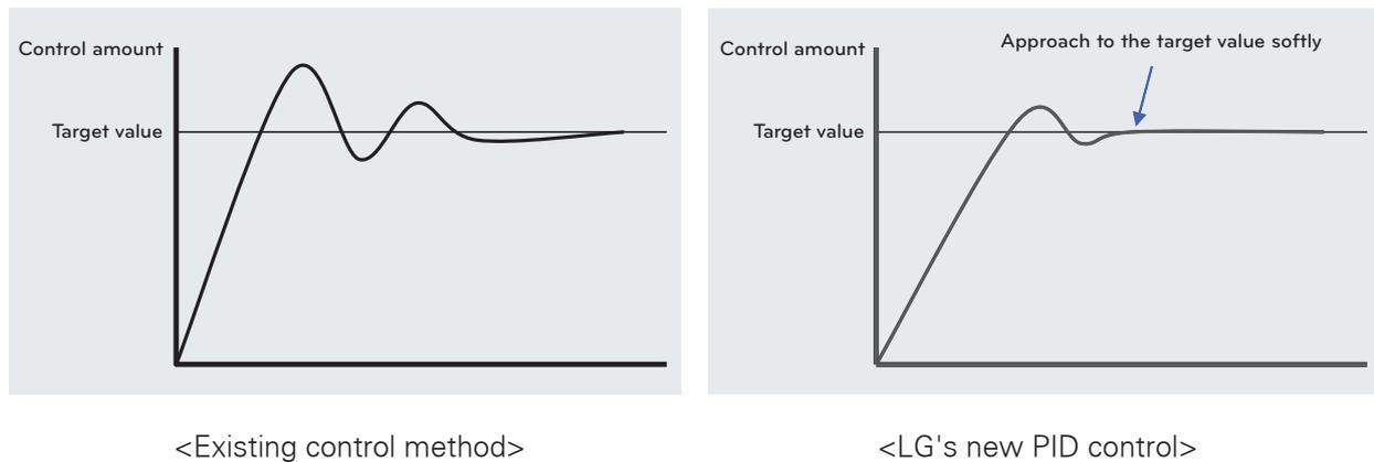
Figure 28. Comparison of control methods
