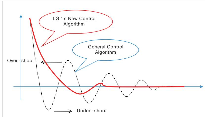
Figure 16. Control algorithm
