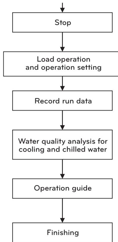
Figure 57. Process from bring-in to test run
