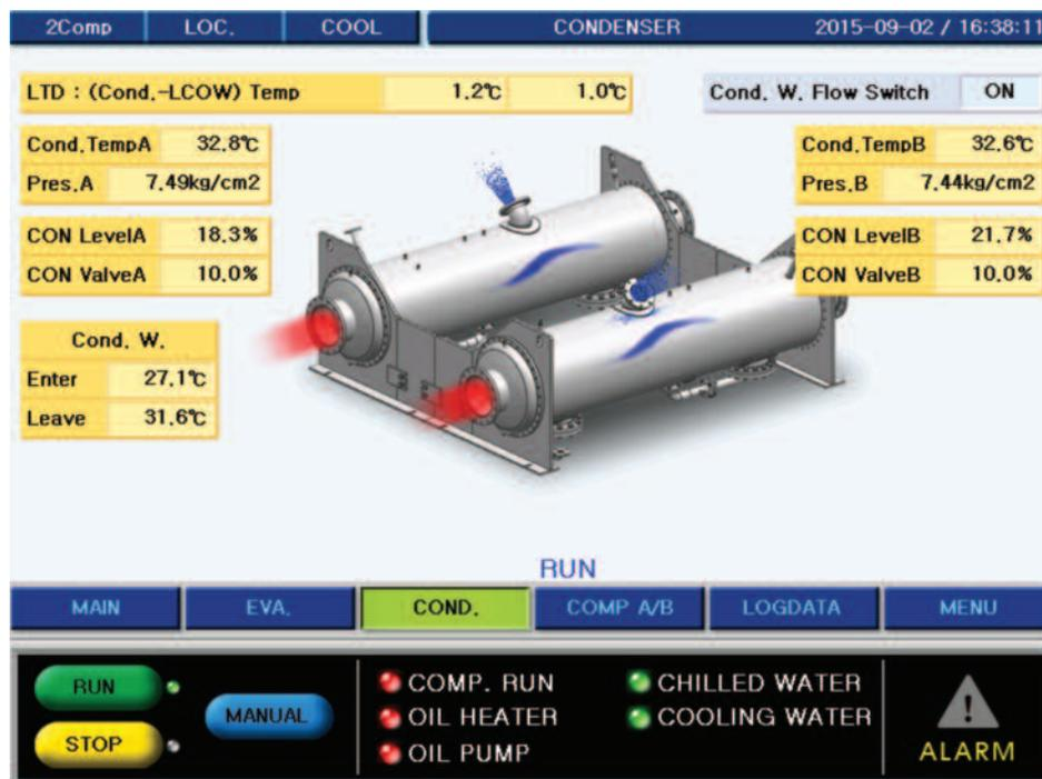
Figure 22. Screen of condenser
