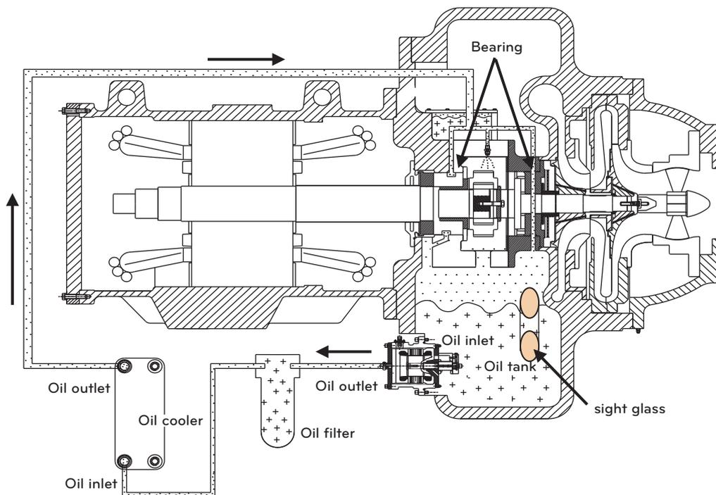
Figure 9. Lubrication cycle
