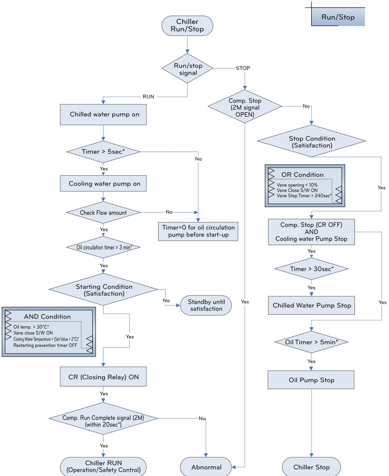
Figure 55. Signal Flowchart
