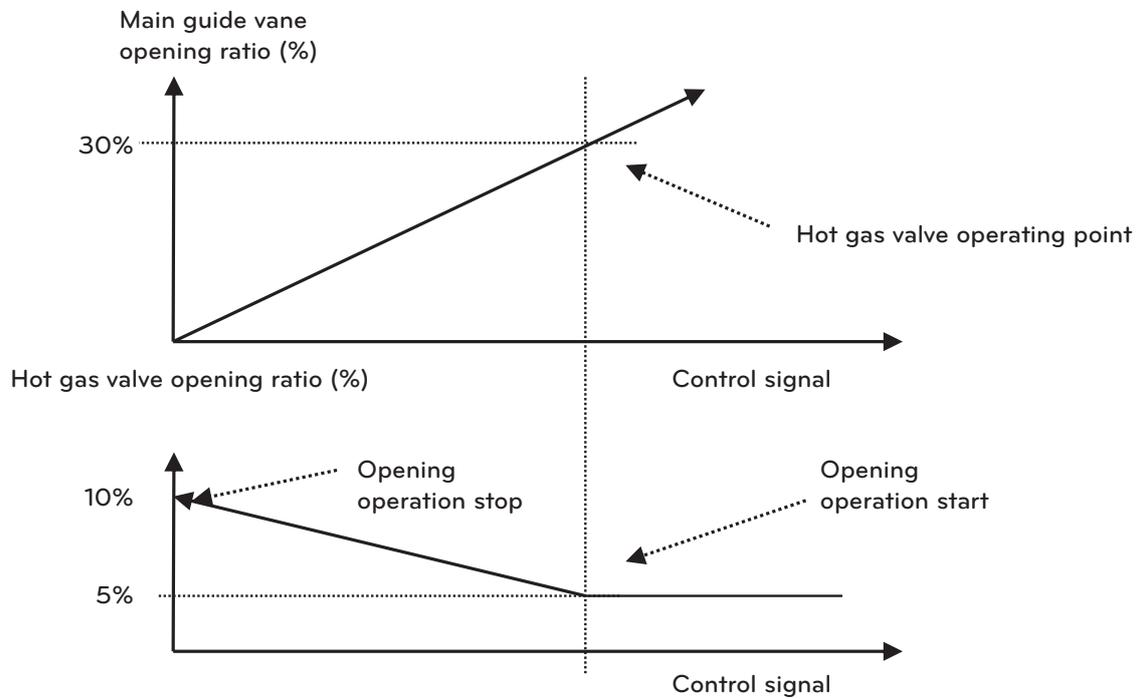
Figure 30. Hot gas valve application diagram
