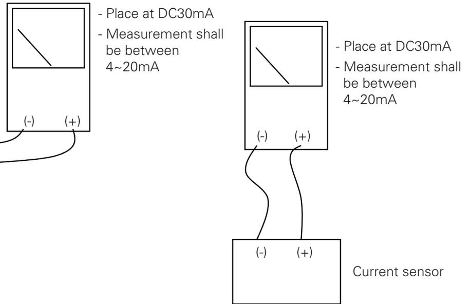
Figure 76. Current Sensor measurement circuit
