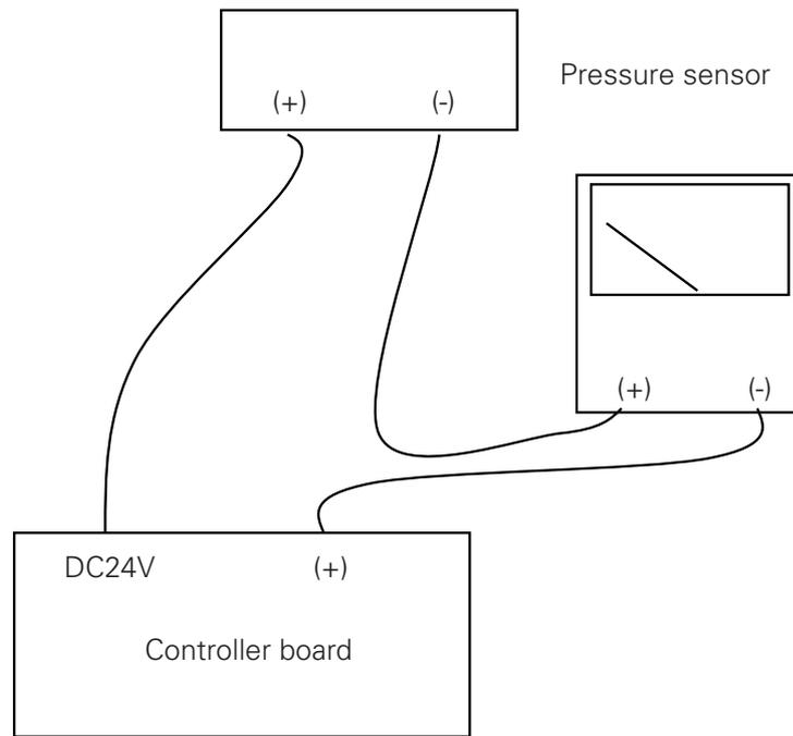
Figure 73. Current Loop Measurement Circuit
