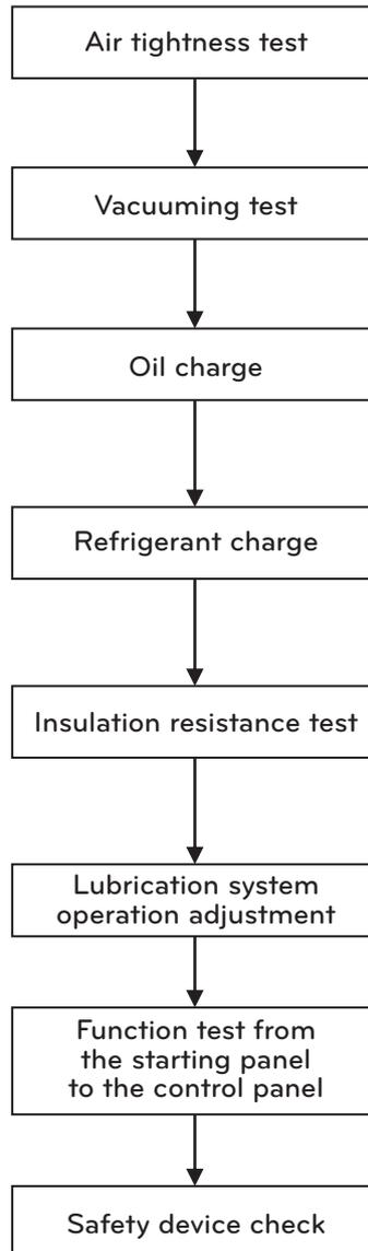
Figure 58. Preparation process for test run
