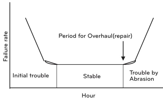
Figure 62. Machine Failure Rate
