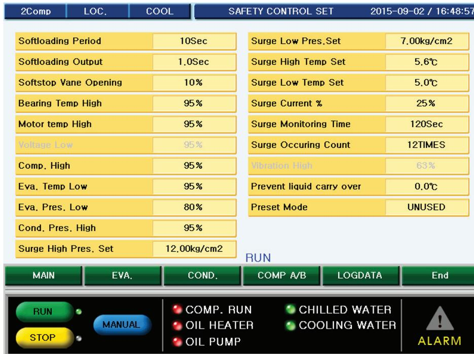
Figure 41. Safety control setting screen
