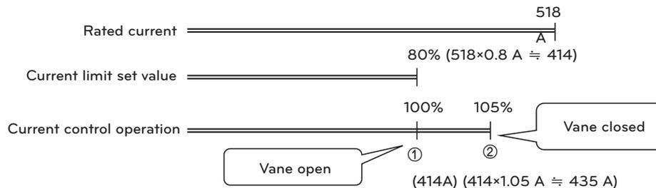
Figure 29. Detailed diagram of current limit
