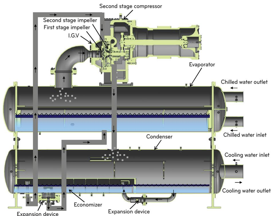
Figure 4. 2-Stage Centrifugal Chiller
