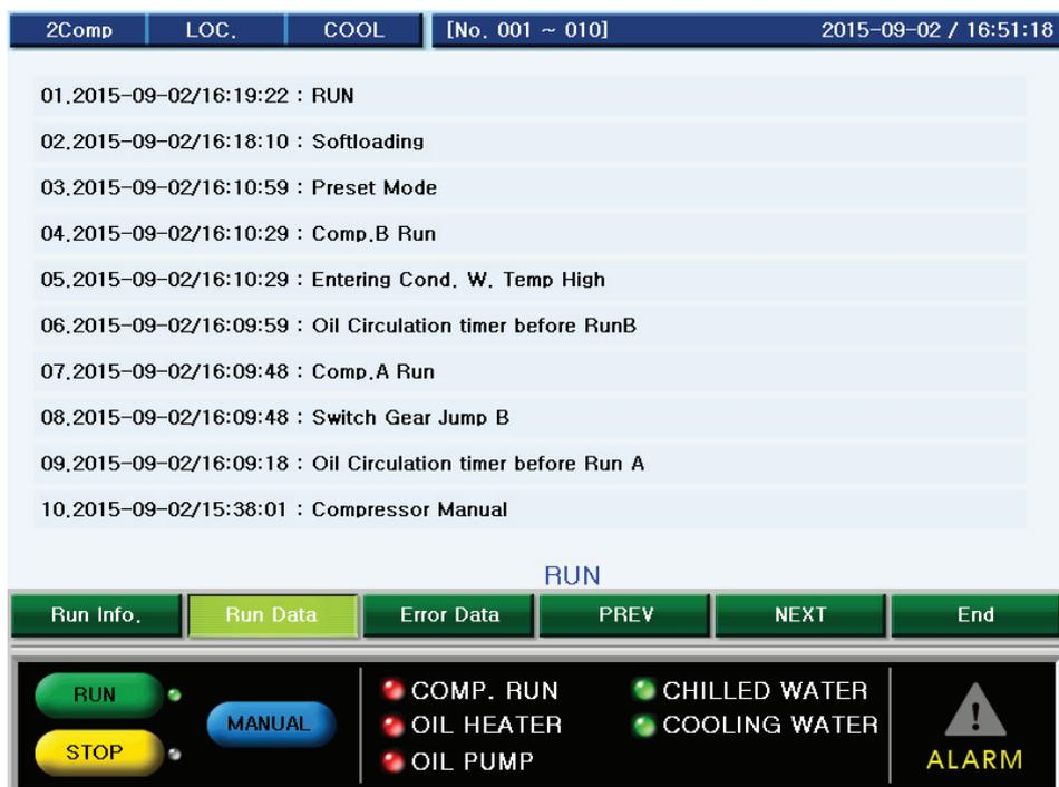
Figure 49. Operation data screen of chiller
