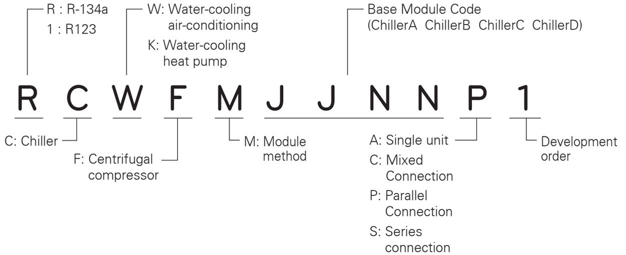
Figure 2. Naming Convention of a Model
