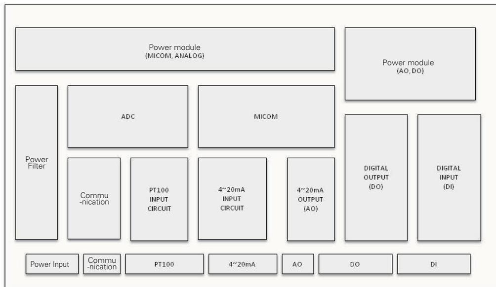
Figure 11. Internal construction of Master/Slave board
