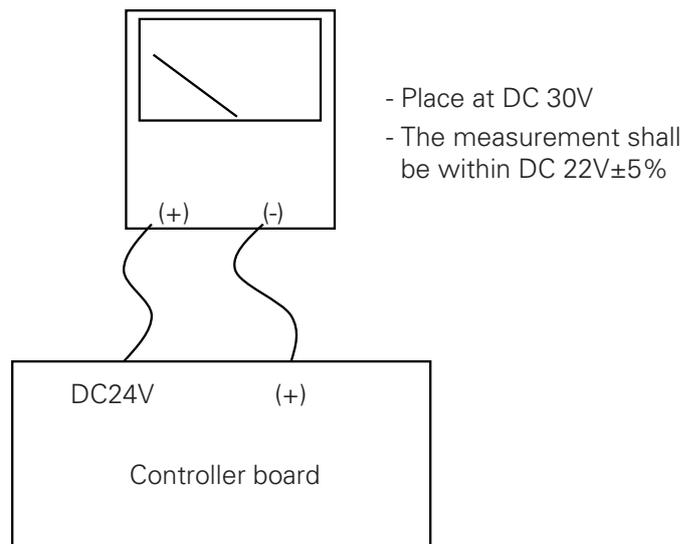
Figure 74. Controller Voltage Measurement Circuit
