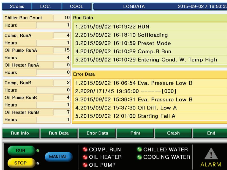
Figure 47. Log data screen of chiller
