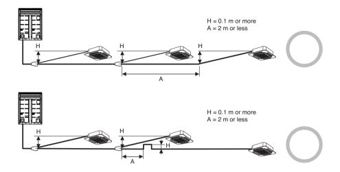
If the indoor unit is located lower than its branch, apply Oil Trap as shown below. Otherwise, the unit may not operate properly.
