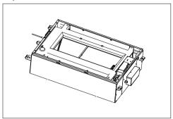
Step4. Assemble control box cover and front panel.
