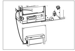
Step2. Assemble PRIP0 with control box cover.
