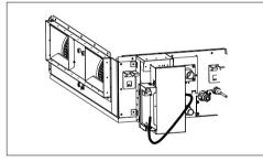
Step2. Assemble PRIP0 with control box cover.
