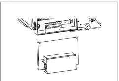
Step4. Assemble control box cover.
