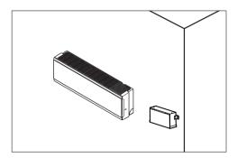
Step2. Connect wires (use a piping or wiring hole) and assemble cover.
