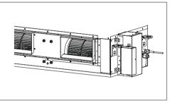
Note: While connecting the PRIP0, attach insulation at the rear of the control box cover where it receives screws as shown in Fig. A.
