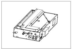
Step4. Assemble control box cover and front panel.
