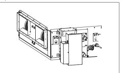
Step4. Assemble control box cover.
