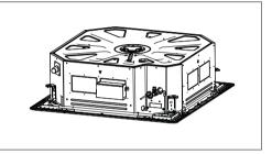
Note: While connecting the PRIP0, attach insulation at the rear of the control box cover where it receives screws as shown in Fig. A.
