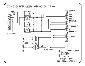
· Connect main lead wires between main PCB and Zone Controller.
