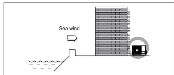
2. In case, to install the outdoor unit on the seaside, set up a windbreak not to be exposed to the sea wind.
