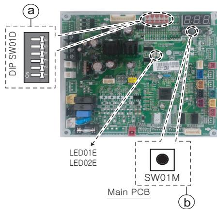
4. After step 3., the LED01E(red LED) and LED02E(green LED) rapidly flickers. When Addressing work is done, green LED is off, else LED(LED01E) stops flickering and lights continuously. Address of indoor unit is indicated on the wired remote control display window. (CH01, CH02, CH03,CH04)
