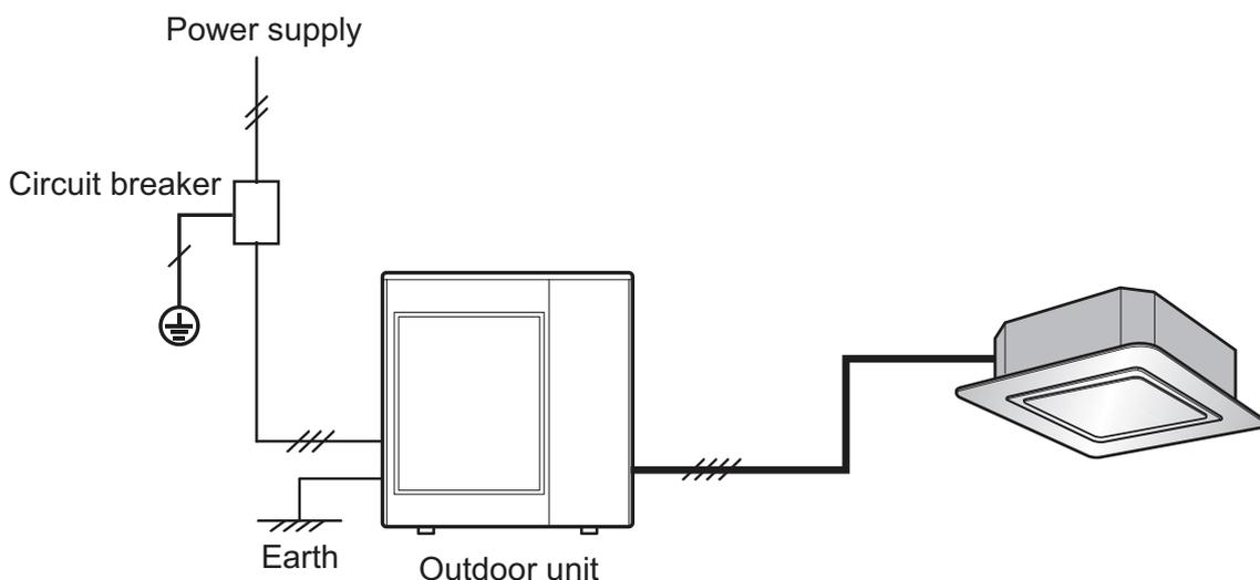
※ This figure is representative example for field wiring. Actual appearance of outdoor and indoor units could be different with installed product.
