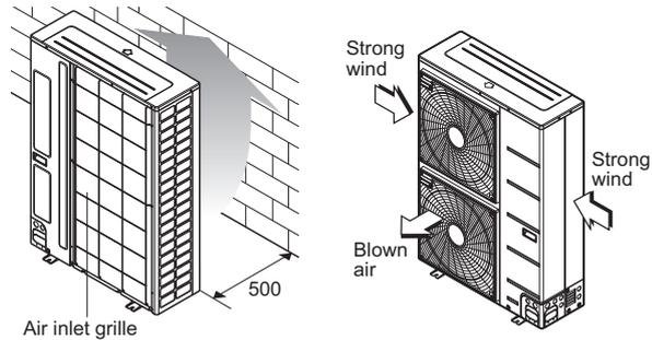
Turn the air outlet side toward the building's wall, fence or windbreak screen.
