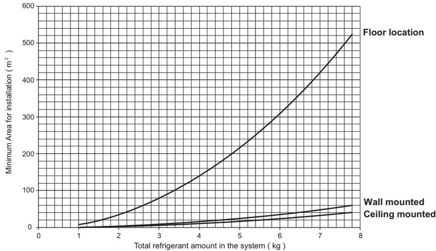
– Total refrigerant amount in the system = factory refrigerant charge + additional refrigerant amount
