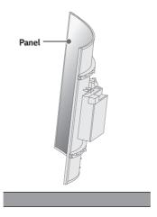
2 When laying down the product, lay a cushion on a flat floor. Put the product on it with the panel of the product facing down.
