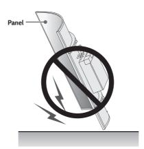
2 If the product is tilted onto the edge of the panel, the panel may be damaged.
