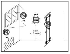
Fig.1 Typical locations for remote controller
